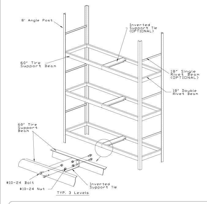
READ BASIC RIVET RACK ASSEMBLY INSTRUCTIONS BEFORE ASSEMBLING
